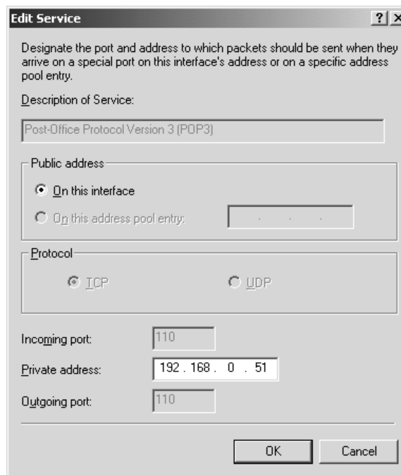
FIGURE 6.52 Assigning an internal address for the port
